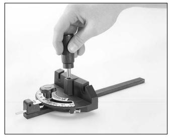
Figure 8. Attaching the miter gauge handle.
